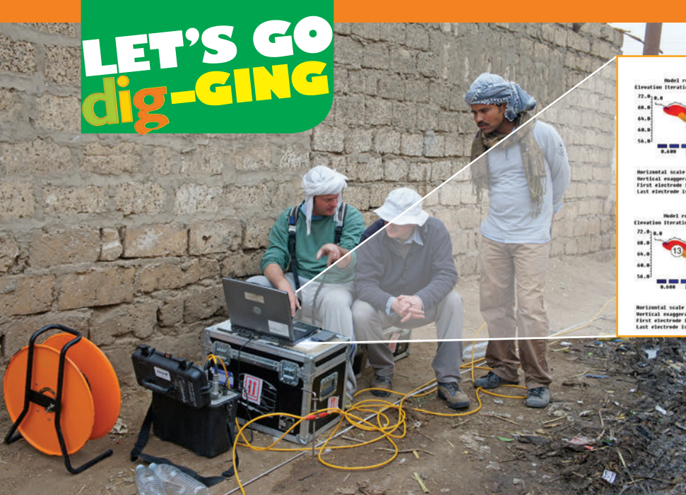
Here's ERT at work: Team members (above) collect ERT results on a laptop. The charts at right above show the results: a section cut through the hippodrome revealing that it has stone structure/foundations.
